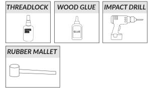
We strongly recommend applying thread lock to the full length of all screws, using Wood glue for the plugs and using an impact drill. Scan the QR code with a phone or tablet to access the assembly video.
